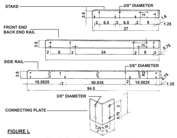
Figure M: Stake Dimensions and Hole Locations
